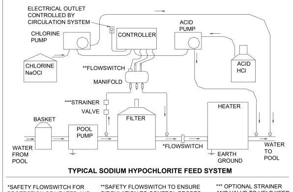
PROTECTION OF HEATER AND TO ENSURE DILUTION OF CHEMICAL INTO POOL.
