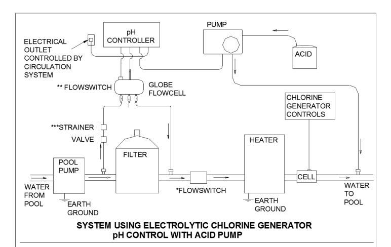
\*SAFETY FLOWSWITCH FOR PROTECTION OF HEATER AND TO ENSURE DILUTION OF CHEMICAL INTO POOL. \*\*SAFETY FLOWSWITCH TO ENSURE CIRCULATION TO CONTROL PROBES AND INDICATOR THAT POOL CIRCULATION IS OCCURRING. \*\*\* OPTIONAL STRAINER AND VALVE TO HELP KEEP MANIFOLD AND PROBES CLEAR OF DEBRIS.
